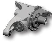
Rear Independent Suspension Split-Case Design
